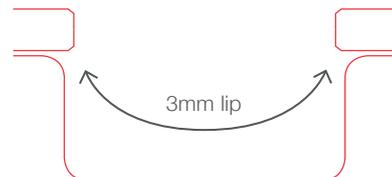
Marbut Stone's standard positioning of undermount sinks as per the above diagram shows a small 3mm overhang of the stone benchtop. If the sink is supplied with fitting accessories (ie; chopping board or bins), the necessary sizing will be applied.
