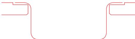
Recessed sinks are always fitted flush with the stone benchtop.
